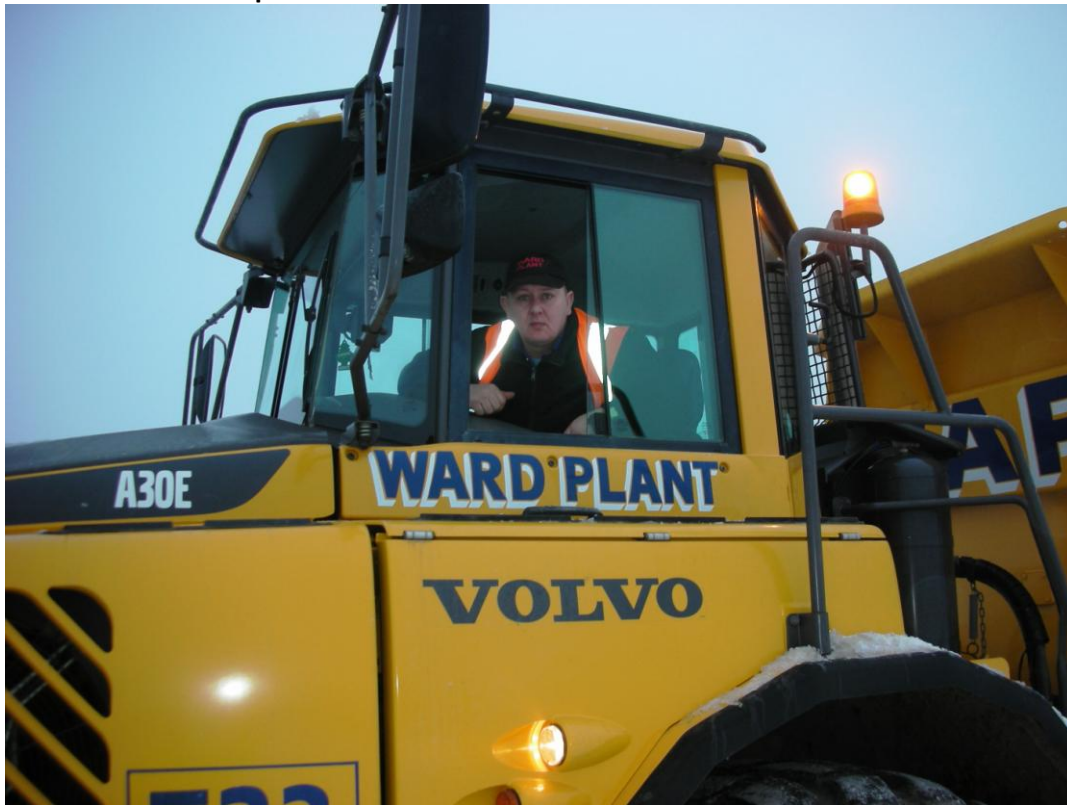
Below – Dougie Rush drives a Volvo A30E articulated dumptruck, hauling material from the excavation area to tip location.
